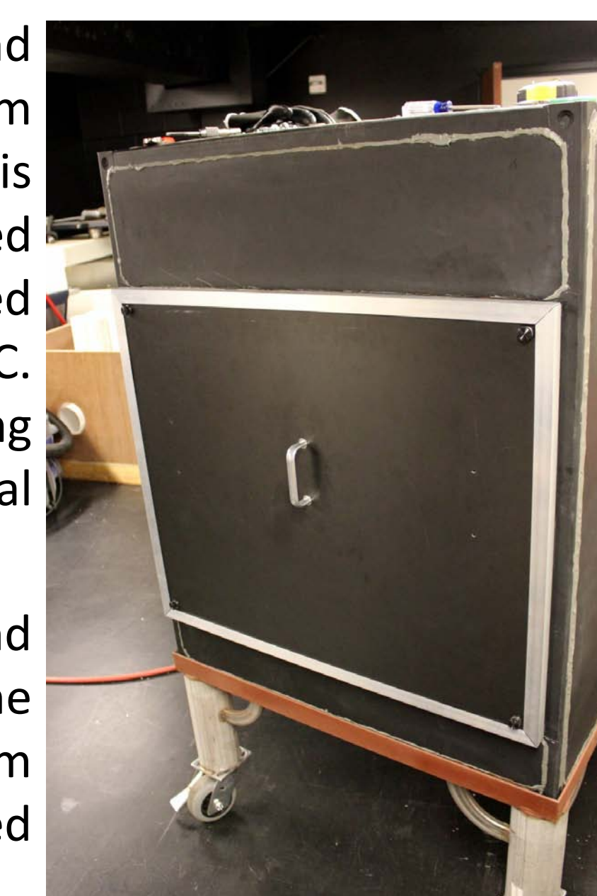
Enclosure door design installed on the enclosure prototype
